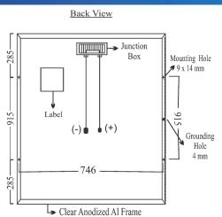
HxWxD 1485X981X40.40 mm
